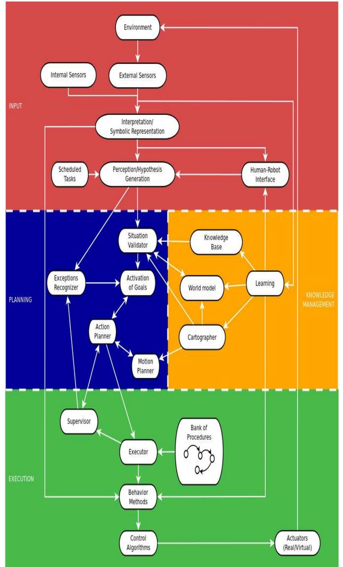
Fig. 1. The VIRBOT System
